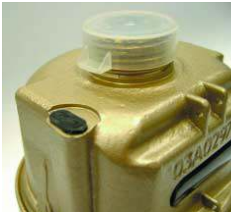
'A' Probe location position under protective plug.
