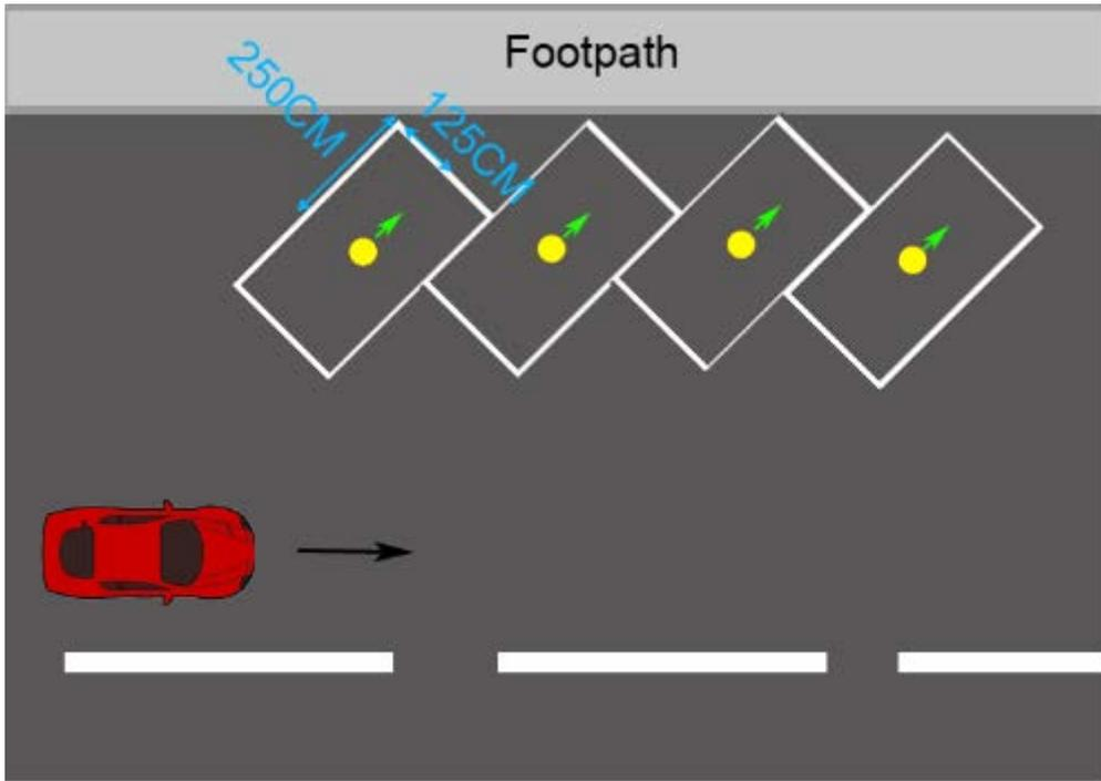
Different Angle parking spot, parallel installation
