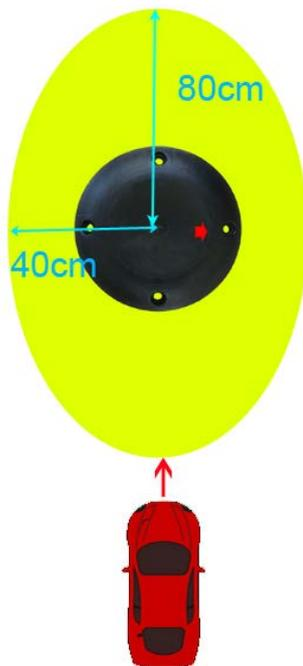
90 degree to the vehicle installation
