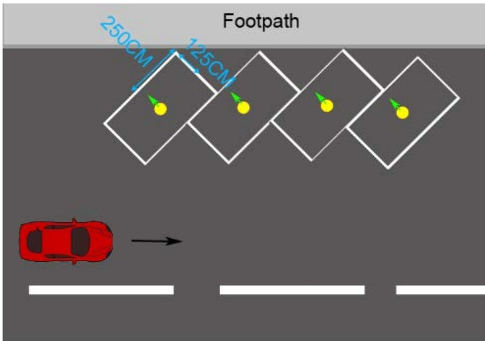
Different Angle parking spot, 90 degree installation
