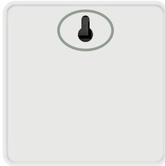
**Caution:** When using a screw for mounting, please make sure that the total length protruding from the wall does NOT exceed 6 mm. Not adhering to this advice might result in physical contact between the screw and internal parts of the sensor causing a loss in range or malfunctioning of the sensor.
