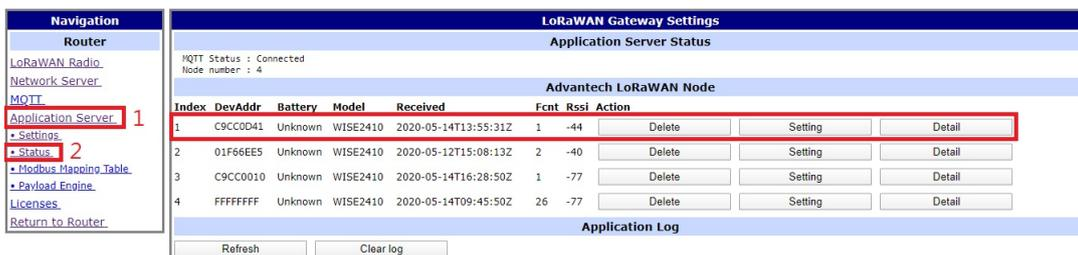
B. Click “Detail”. The gateway will help to pre-parsing the data payload if the “App Arguments” input correctly.
